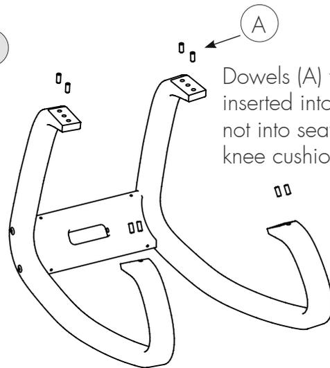
Dowels (A) to be inserted into the runners, not into seat or knee cushions.
